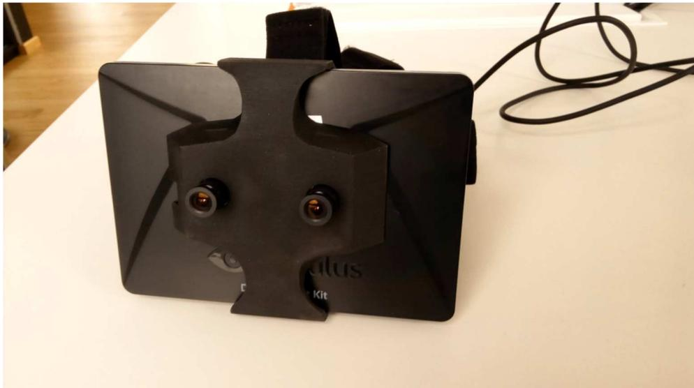
Figure 9: Virtual reality headset with front mounted stereo camera
