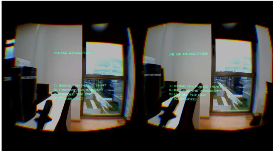
Figure 56: Stereo display with direct video feed and overlaid text
