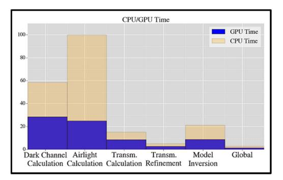
Figure 3 – Dark channel dehazing performance.
