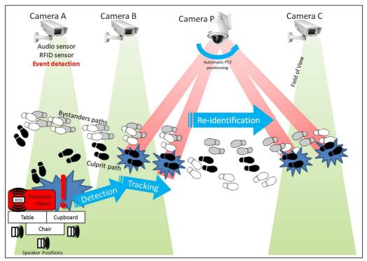
Figure 2 – Testing scenario scheme.
