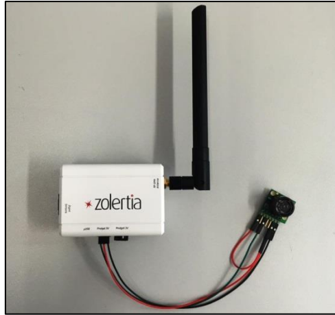
Figure 20: Node: pair ultrasonic sensor + Z1 source mote
