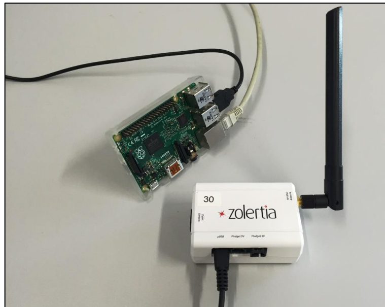
Figure 21: Raspberry Pi 2 + Z1 sink mote
